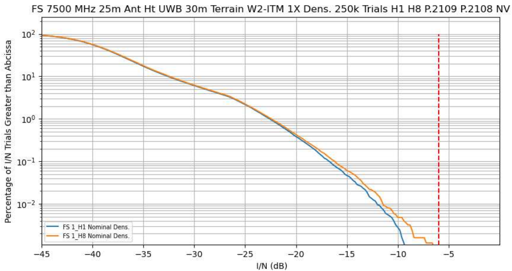
Figure 25. Fixed Service I/N with 30 m Terrain Height with FS antenna height of 25 m. H1 and H8 UWB antenna heights
