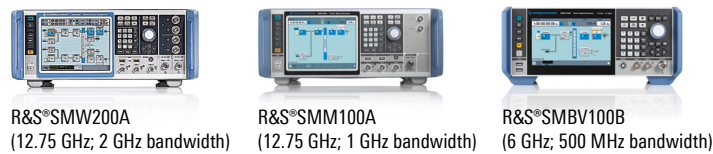
Figure 9-3: Rohde & Schwarz signal generators and signal analyzer for UWB applications
